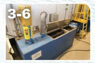
First of three water rinses, ending in pure reverse osmosis water. Finishing with a dried-in-place aluminum sealer.
