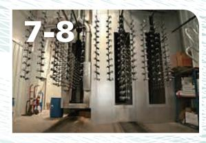
A 200 MPH air blast removes water drops from the pre-treated aluminum. A convection oven completes the dryoff process.
