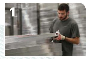
The raw premium-grade aluminum is inspected to be free of blemishes and is not exposed to the outdoor elements.
